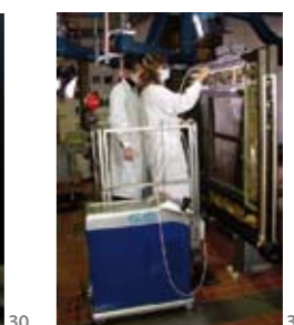
33 e 34. Portable fibre optics sensors applied on paintings for pigments analysis.
