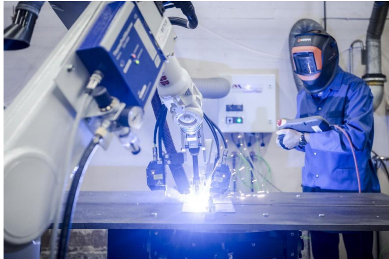
Figure 9 - Welding robot at LUT
