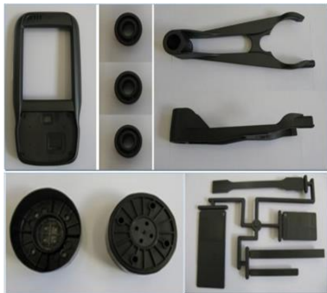
Figure 14 – Examples of polymer/graphene nanocomposites prototypes produced by ISOF-CNR and SMEs located in the Emilia-Romagna region.
