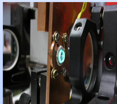
Yb:YAG ceramic element emitting laser radiation. Turquoise fluorescence is due to the pump up-conversion
