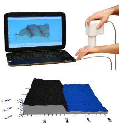
Palm-sized 3D digital microscope and application examples: a) examination of skin, b) observation of a painted surface during laser cleaning.
