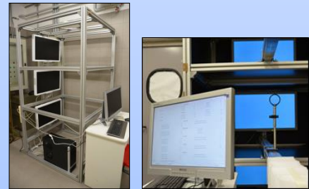
Dynamic star-field simulator particular of control interface and collimator.
