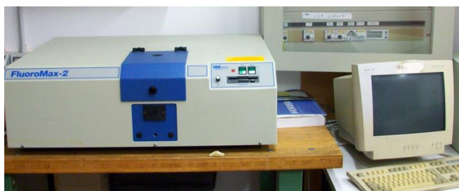
Fig. 3. Horiba FluoroMax-2 spectrofluorimeter.
