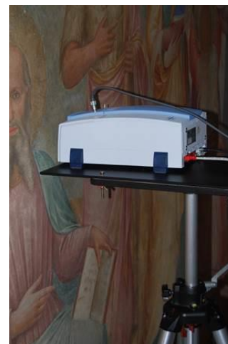
Fig. 1. Alpha Bruker Optics FT-IR Spectrophotometer at the San Marco Museum, Florence.
