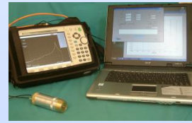
The SUSI® system detects moisture and soluble salts
