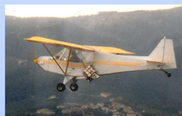
X-band radiometer adapted for an ultralight airplane
