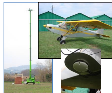
GNSS_R sensor installed on ground and on an ultra-light aircraft (detail of the GNSS antenna)
