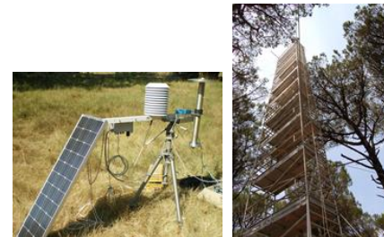
Ground measurement instrumentation and eddy covariance flux tower (in collaboration with JRC- Ispra).
