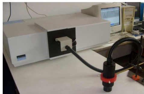
Fig. 2. Perkin Elmer Lambda 900 Spectrophotometer equipped with the external integrating sphere.
