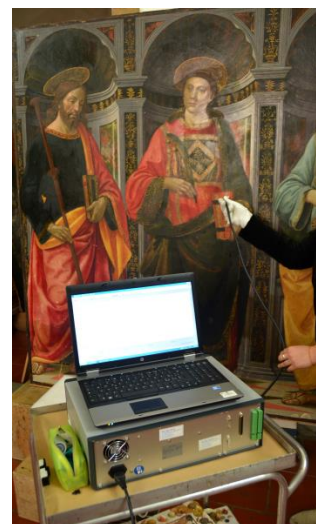
Fig. 1. FORS device during a diagnostic campaign on the painting Santo Stefano fra i Santi Jacopo e Pietro by Domenico Ghirlandaio, Galleria dell'Accademia, Florence
