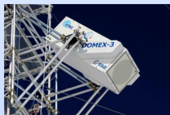
L-band radiometer installed on the US tower at Concordia Station, Antarctica
