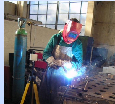
Measurement of electric and magnetic fields close to an industrial welding station
